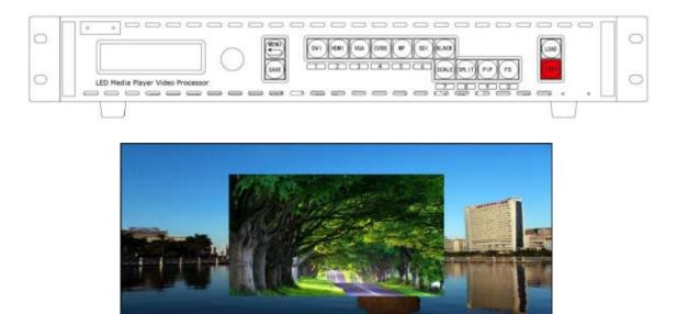
Press SCALE button to change layer B size and position.
